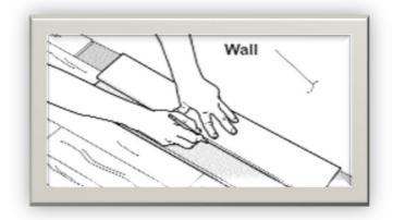
The last row (possibly the first row) plank width should be no less than  $50 \text{mm} (2^{\circ})$  on the long seam. Remember to allow for a gap of  $10 \text{mm} (3/8^{\circ})$  to the wall.
