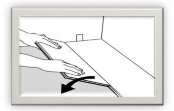
Cut a piece that is a least 5.9" or 150mm shorter than the first plank to start the second row or use the cut off from the previous row, keeping in mind the length requirements above.
