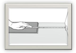
The last piece in the row should be cut to length while maintaining the 10mm expansion gap along the perimeter of the room.
