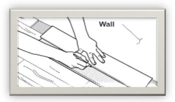
The last row (possibly the first row) plank width should be no less than 50mm (2") on the long seam. Remember to allow for a gap of 10mm (3/8") to the wall.
