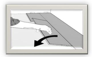
To install the remaining planks in the second row, first align the long edge tongue into the groove of the previous row at a shallow angle. Slide the piece to the left until the piece meets the previously installed piece.
